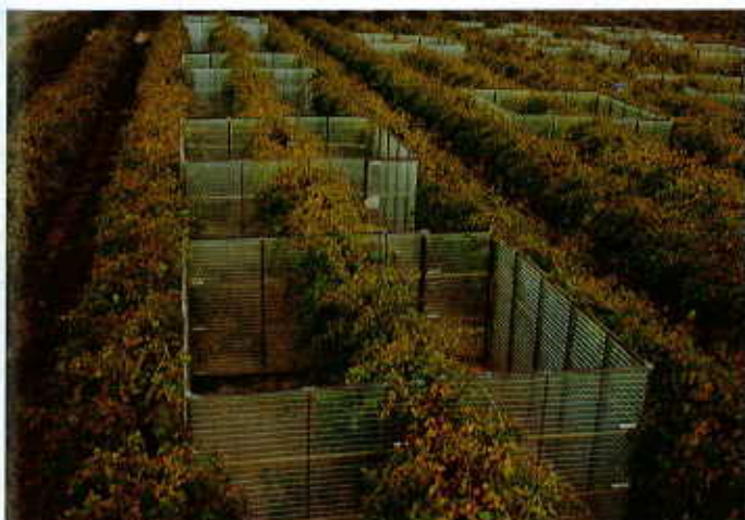
Figure 1. Open-top chambers in a 17-year-old Shiraz vineyard, used for applying the treatments described in Table 1. Chamber dimensions are 5.5m x 8m x 2.4m (LxWxH).
