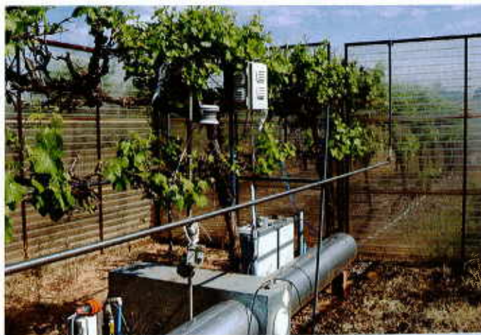
Figure 2. Inside an elevated CO 2 and temperature treatment (eCO 2 +eTemp) open top chamber. CO 2 emitters and fan-assisted electrical heaters are located below the vines' canopies.
