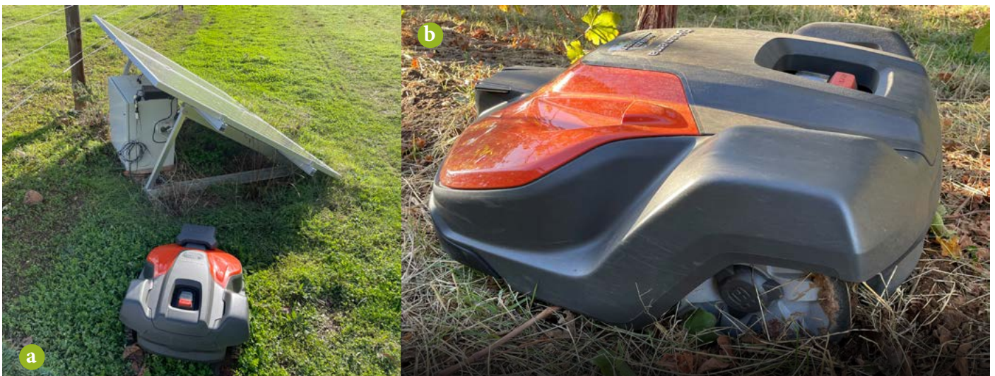
Figure 5. Husqvarna Automower (a) charging using off-grid solar-battery station, and (b) stuck with rear wheels slipping
