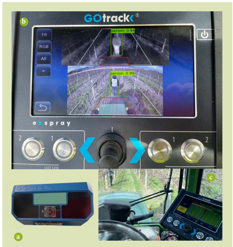
Figure 3. GOtrack (a) obstacle detection camera (b) live camera view testing object recognition, and (c) cab view after detecting a person and stopping during actual operation (safety driver in place)
