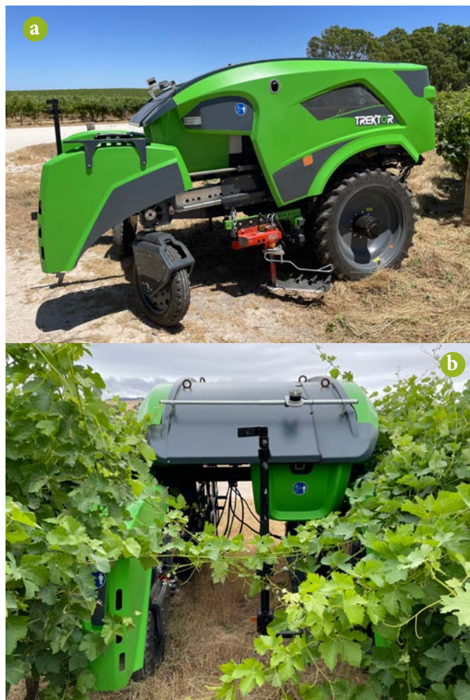
Figure 4. SITIA Trektor with mid-mount blade weeding tools (a) turning into the next row, and (b) bump sensors activated by the sprawling canopy
