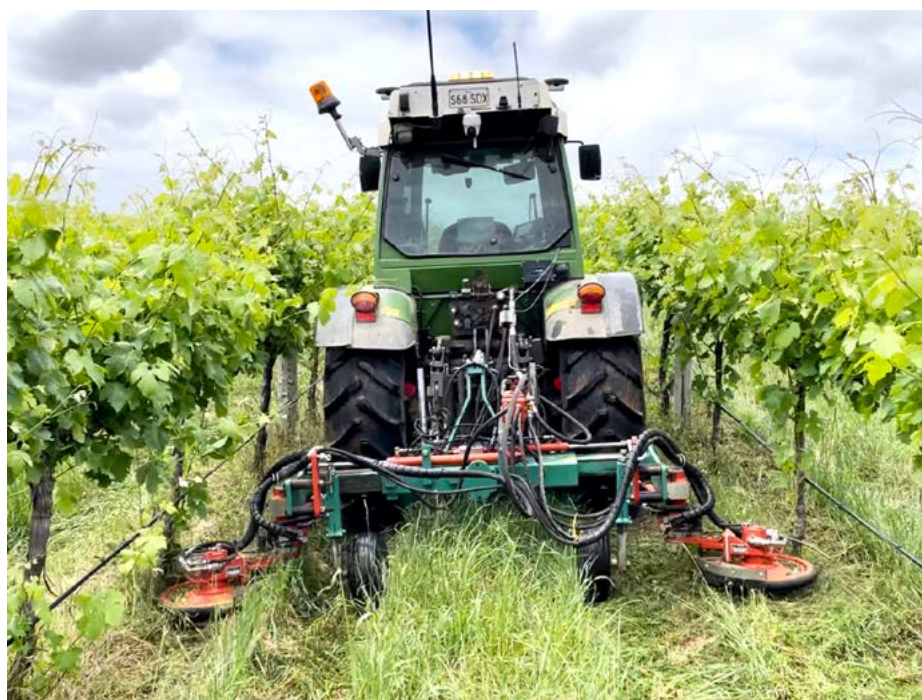
Figure 2. Autonomous under-vine mowing using the tractor fitted with the GOtrack autonomy-kit
