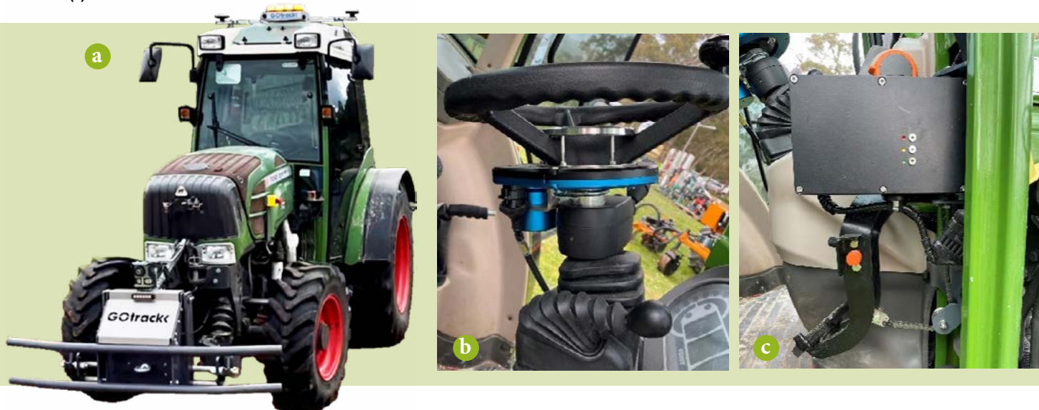
Figure 1. Fendt 211P Vario tractor with GOtrack autonomy-kit fitted: (a) with bump sensor, stop buttons, LIDAR and GNSS-RTK antenna bar (b) Steering-wheel drive (c) Brake drive
