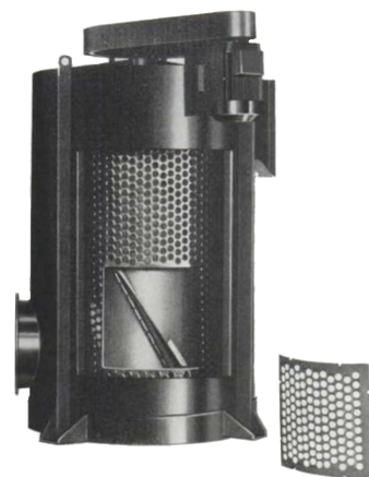
Figure 13. Vertical centrifugal beater crusher-destemmer with feed on the bottom left, image c. 1970s
